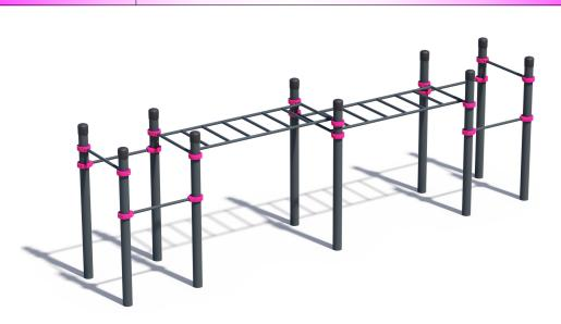
The complex consists of ten vertical columns, six crossbar with the length of 800mm and two horizontal monkey bars of different height. Length of the monkey bar 1952mm, width 800mm, distance between crossbars is 274mm. The complex is secured together with aluminium clamps.
